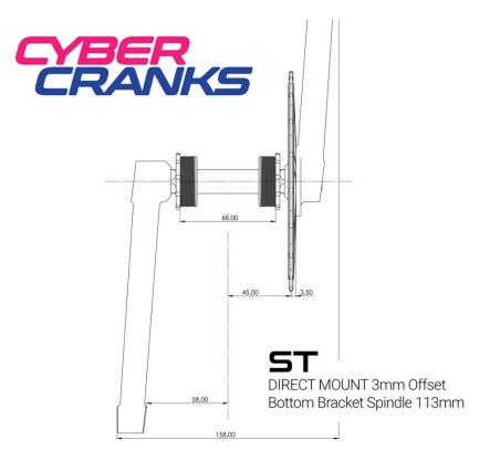
The square taper should be clean and free of grease. To fit the cranks, use an 8 mm Allen key and tighten the screw to max. 30 Nm. A higher tightening torque can damage the integrated puller. The square of the inner bearing should be clean and free of grease. After approx. 50 km of riding, please check the fit of the crank bolt and retighten if necessary. The crank bolt is held in place by a replaceable cover cap. To remove the cover cap, please use a face wrench with two pins.
