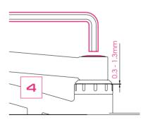
Finally, the left-hand crank including the screw is fitted onto the shaft. The fastening screw must be tightened with an 8mm hexagon socket and 25 Nm. After tightening the screw, a gap of between 0.3 - 1.3 mm should be visible. It is recommended to secure the screw with a medium-strength thread-locker (e.g. Loctite 243).
