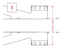
First, install the bottom bracket according to the manufacturer's instructions. Then measure the width of the installed bottom bracket. The width must be between 92.5 - 95.5mm. For 68mm wide frames, a spacer of 2.5mm should be used between the frame and the bottom bracket shell.
